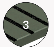
3 GROOVE WITH EPOXY FILLING
